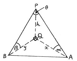
In the above diagram of a triangular pyramid, AQ = x, BQ = y, PQ = h,  $\angle APB = \theta$ ,  $\angle PAQ = \alpha$  and  $\angle PBQ = \beta$ . Also, there are three right-angles at Q.
