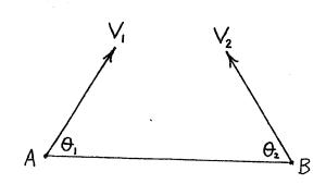
Two particles  $P_1$  and  $P_2$  are projected simultaneously from the points A and B, where AB is horizontal. The motion takes place in the vertical plane through A and B. The initial velocity of  $P_1$  is  $V_1$  at an angle  $\theta_1$  to the horizontal, and the initial velocity of  $P_2$  is  $V_2$  at an angle  $\theta_2$  to the horizontal.
